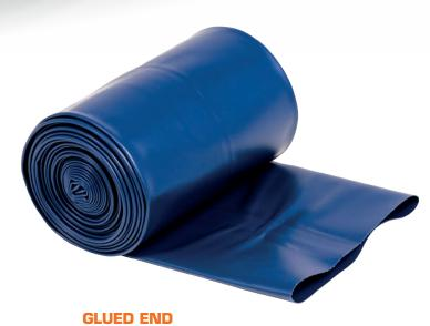
The glued end is used on installations where you don't want, or have the possibility to cut away the far end of the liner. For example from the house out to the main. The Omaplata hose is used as an extension of the liners coating that protrudes the liners far end, and is retracted after curing. This leaves the liner open and there is no need for further work.
