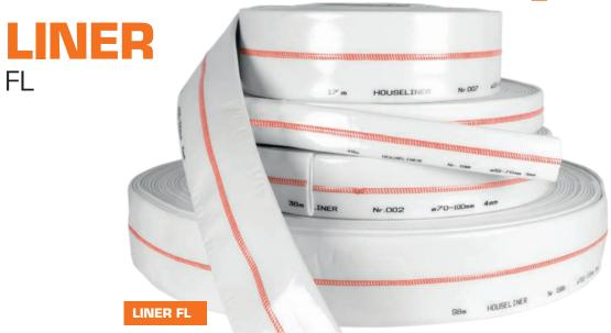
Houseliner FL is your go-to liner. It comes in a variety of sizes and thicknesses to suite your needs. From DN3O all the way to DN4OO. Wall thickness from 2,5 to 5mm depending on your choice of liner. Made from 100% PES fiber with a TPU coating. Suitable for ambient, UV or hot water curing up to 80°C.
